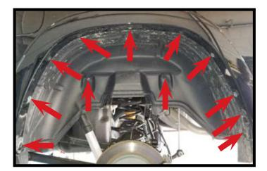
2. Remove both wheel well liners by removing 12 screws from the inside of each rear wheel.
