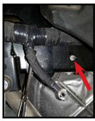
**9.** On the drivers side, temporarily remove the nut from the wiring stud so that the bracket can go behind the wire harness and be placed tight to the frame. Replace wiring nut when bracket is installed
