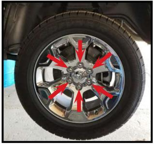
**1.** Remove the rear tires by either placing the truck on a hoist, or jacking the rear up.
