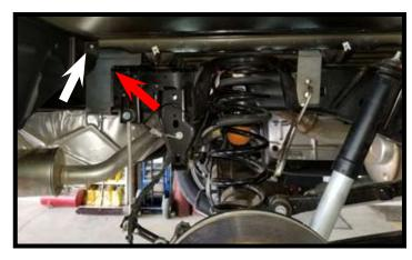
NOTE: In some cases, to aid in the install of the rear brackets, temporarily remove the screw maked by a white arrow.
